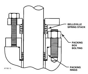
Figure 7. Live Loaded PTFE Packing
