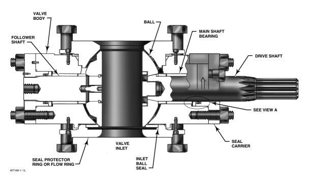
Figure 2. Sectional View of Design V250 Valve
