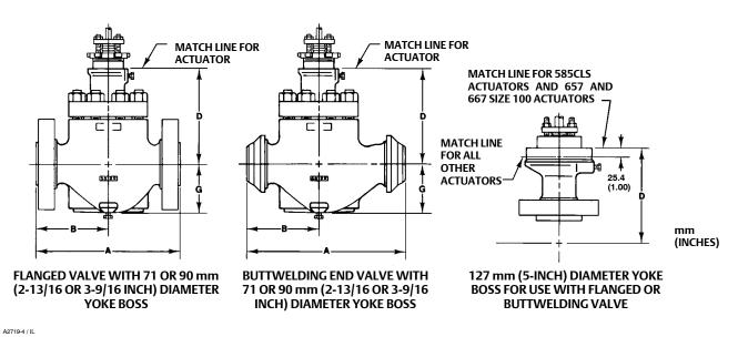
Figure 23. NPS 1-1/2 x 1 through 6 Globe Valve Dimensions with Standard Bonnet (also see tables 21, 22, and 23)
