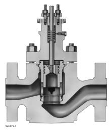
Control Flexibility—Special cage characterization (standard, Whisper Trim, or Cavitrol trim) can be supplied to satisfy almost any combination of flow and noise or cavitation abatement. Cage characterization and efficient flow passages provide close control for low flow, high pressure drop conditions as well as high flow, low pressure drop conditions. A choice of actuator styles allows wide selection of power and control capabilities.
