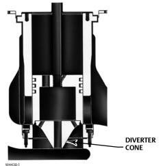
DIVERTER CONE VALVE PLUG USED IN BOILER FEEDWATER SERVICE FOR FLOWING  $\Delta P$ > 1000 PSI (69 BAR) AND IN OTHER APPLICATIONS FOR FLOWING  $\Delta P$ > 138 BAR (2000 PSI) OR FOR WHISPER TRIM III LEVEL A, B, OR C CAGES
