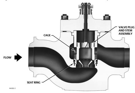
Figure 14. Sectional of NPS 20 Fisher EHD Control Valve Assembly
