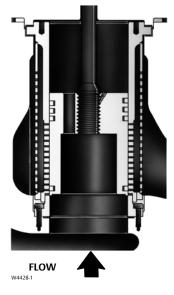
Figure 12. Diverter Cone Valve Plug Used in Fisher EHD and EHT Valves (NPS 8 through 14 Globe Valves, Flow Up Only)
