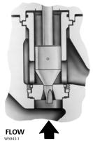
Figure 7. Diverter Cone Plug Used in NPS 6 Fisher EHD and EHT Valves (Flow Up Only)
