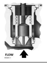
Diverter cone valve plug used for flowing  $\Delta P$ > 207 bar (3000 psi) or for Whisper Trim III Level A, B, or C cages.
