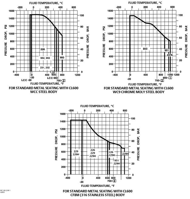
Figure 6. Temperature and Pressure Drops for Typical Trim Used in Fisher EUD, EWD, EUT, and EWT Valves
