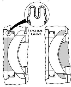
FORWARD FLOW SHUTOFF REVERSE FLOW SHUTOFF 4283375-A
